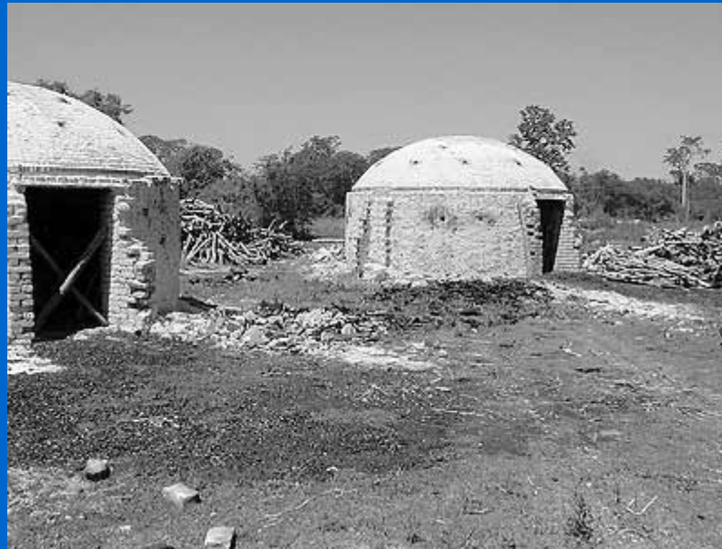
Fig. 2. Traditional industrial charcoal production: a Brazilian-type brick kiln in Cuba
